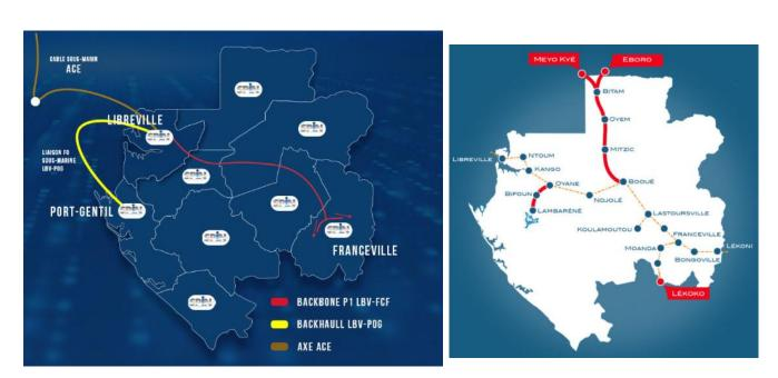
Figure 36 Broadband fiber optics transport network routes phases 1 and 2
